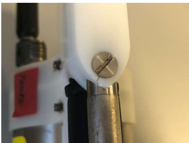
Cracked support of the bar which protect the conductivity cell and dirty pump-tubes circuit.
