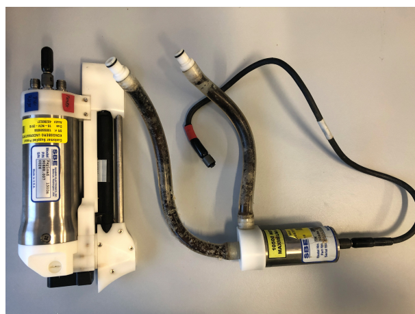
Cracked support of the bar which protect the conductivity cell and dirty pump-tubes circuit.
