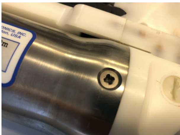
Damaged/scratched screw and pry slot.
