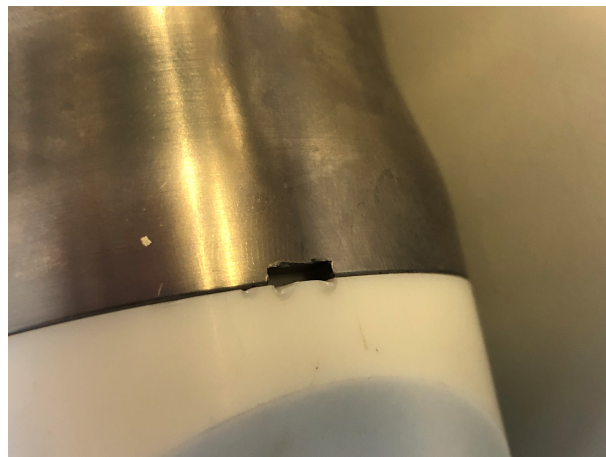
Damaged/scratched screw and pry slot.
